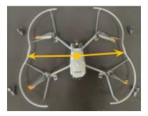
Install the four 3D printed feet on the drone's front left, front right, rear left, and rear right.
